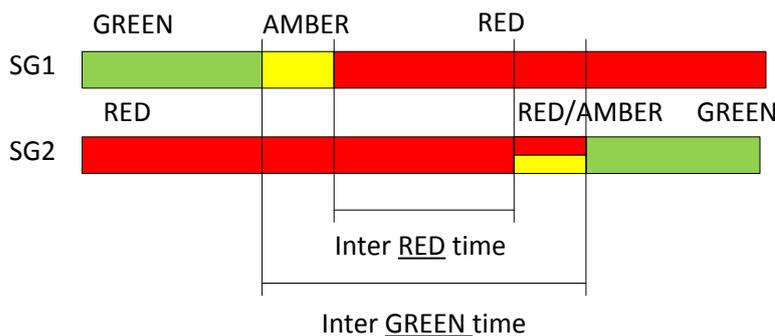
Figure 6 Clearance timing
