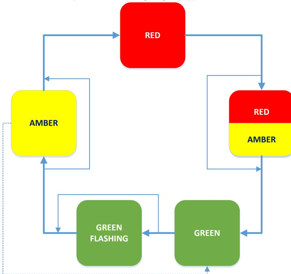
Figure 5 Signal group control-state transitions (Control)
