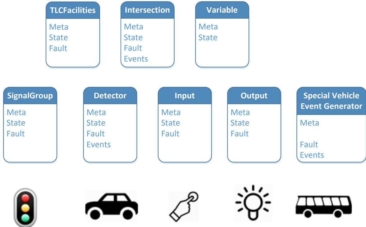
Figure 9 Top-level objects for the TLC-FI
